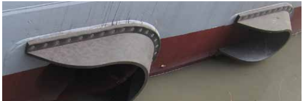
Photo of caps installed on a ship's side
