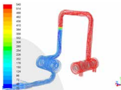
Flow pathlines through the exhaust gas system and colored by temperature
